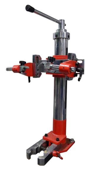
SuperATV strongly recommends using a Spring Compressor, not included, when removing and installing Springs.
