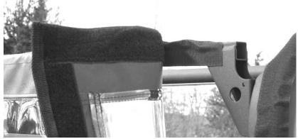
2. Next place the two 22" adhesive Velcro strips down the side bars. You will need to cut the Velcro so it adheres to each part of the frame. See photos below.
