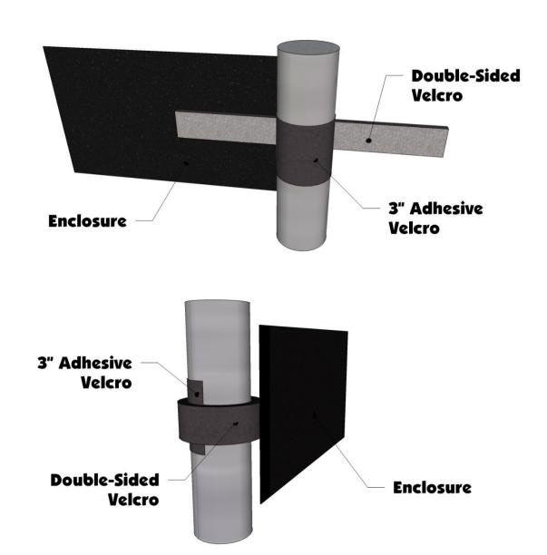
4. The bottom corner of the door is held in place by 6" and 32" adhesive Velcro strips. The photo below shows the proper placement.
