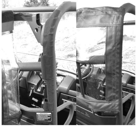
3. The bottom of the Rear Window is held in place by the 42" adhesive Velcro strip. The strip goes across the bottom on the plastic from one side to the other. The adhesive strips go on the bottom of the overhang on the plastic. The photos below show what it should look like.
